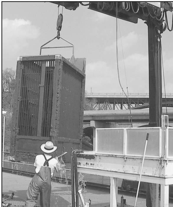
Baskets at the Fishway are lifted daily. Here the catch is emptied into a sorting table.
