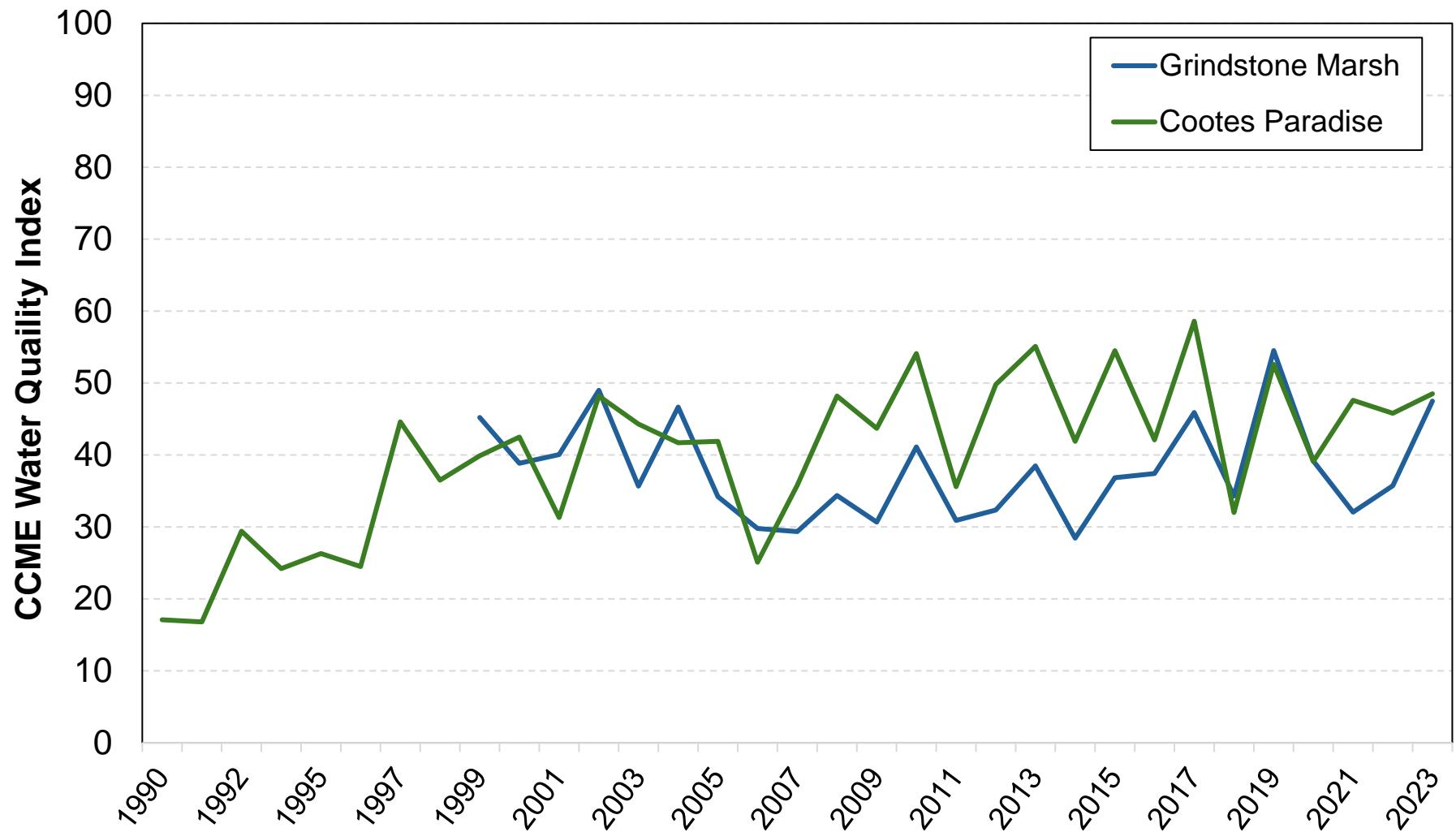
CCME water quality index score centre stations / HHRAP delisting station (GC-1, CP-2) using parameters of Nitrate-N, ISS, TSS, Total Phosphorus, *E. coli*, and dissolved oxygen. Scores >90 = appropriate clean water.
